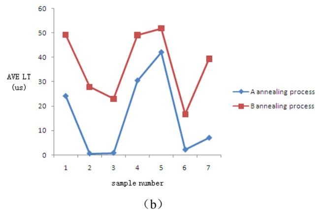
Figure 3:(a) The lifetime of different oxygen content (annealed by the same process); (b) The lifetime of the same silicon slice annealed by different process.
