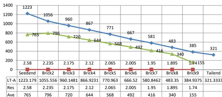
Figure 4. Oxygen concentration and MCL for LONGi's p-type ingot sample.
